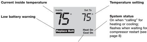
If flashing, compressor protection is engaged (see page 8)
