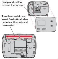
Install fresh batteries immediately when the **REPLACE BATT** warning begins flashing. The warning flashes about two months before the batteries are depleted.
