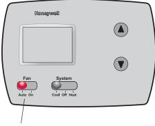
Set FAN switch to choose whether the fan runs continuously or only as needed.
